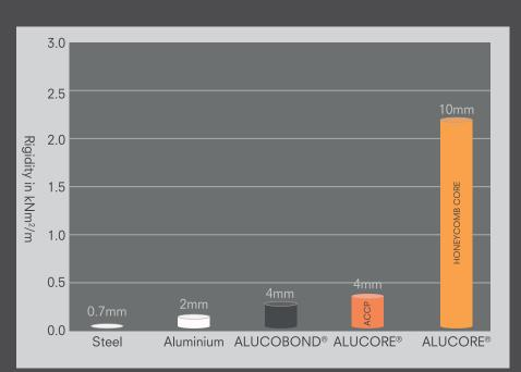
The graph illustrates the rigidity of different materials while keeping the weight identical.
