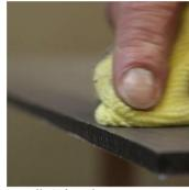
Immediately wipe away any excess that appears on the panel surface. Failure to do so will result in stain that cannot be removed.
