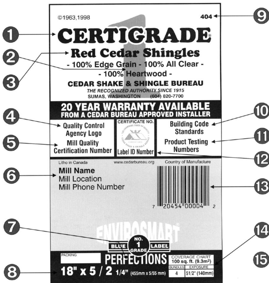
Figure 1. Information on a Certi-Label™: 1) “Certi” brand name; 2) Product grade; 3) Product type; 4) Independent third party quality control agency; 5. Compliance with total quality processes; 6) Manufacturer; 7) Industry product description; 8) Product dimensions; 9) Cedar Bureau label number; 10) Building code compliance numbers; 11) Product performance tests passed; 12) Label identification number; 13) UPC code; 14) Coverage showing the number of bundles/100 square-foot and recommended exposure; 15) Application instruction on reverse side. Used with permission from Cedar Shake & Shingle Bureau, New Roof Construction Manual .
