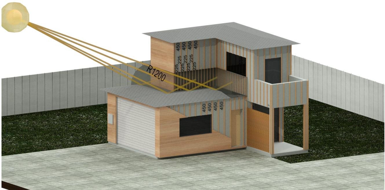
Any cladding which is above a metal roof requires the battens to be installed at maximum 225mm centres for any area of cladding which is within a 1.2m radius of the metal roof (in any direction).
