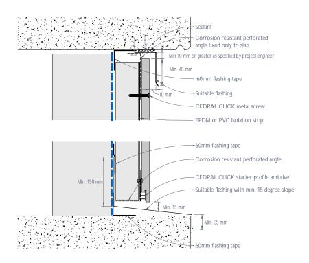
Figure 26: CEDRAL CLICK junction with exposed concrete slab or beam - Cladding recessed
