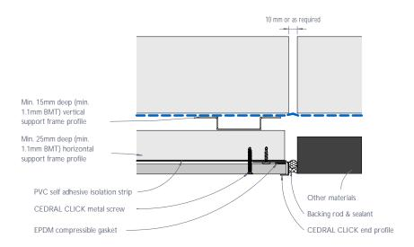
Figure 6: CEDRAL CLICK vertical control joint - Detail 3
