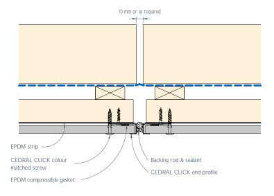
Figure 6: CEDRAL CLICK vertical control joint - Detail 3
