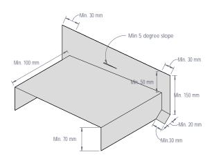
Figure 36: Corrosion resistant saddle flashing
