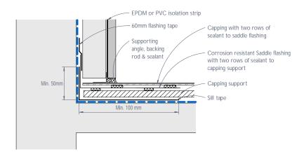
Figure 36: CEDRAL CLICK parapet junction - Section
