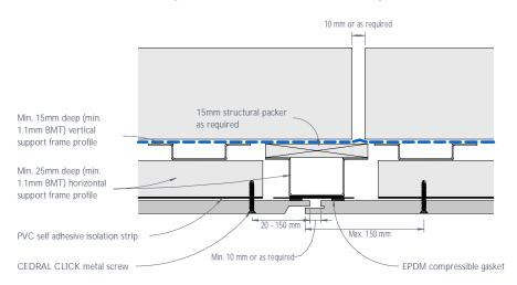
Figure 4: CEDRAL CLICK vertical control joint - Detail 1
