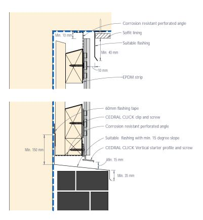
Figure 22: CEDRAL CLICK junction with other materials, eaves or the like - Recessed detail
