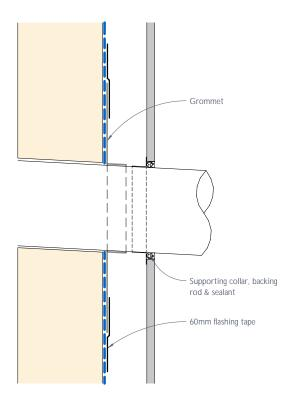
Figure 31: Pipe penetration - Section
