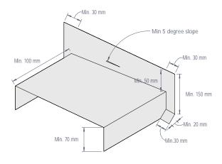
Figure 38: Corrosion resistant saddle flashing
