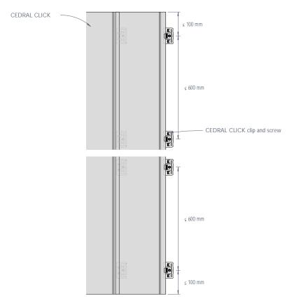
Figure 1: CEDRAL CLICK fixings arrangement - Elevation
