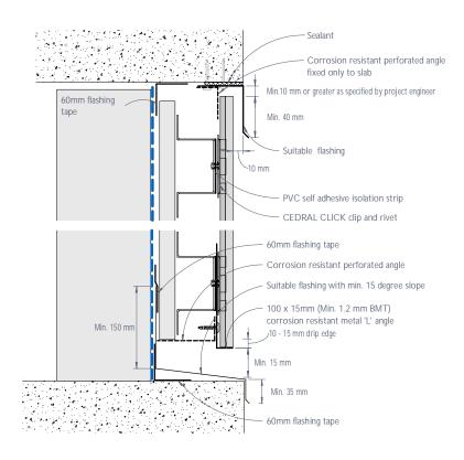
Figure 22: CEDRAL CLICK junction with exposed concrete slab or beam - Cladding flush
