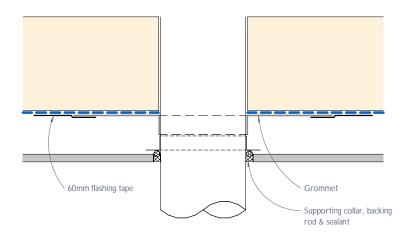
Figure 29: Pipe penetration - Plan view
