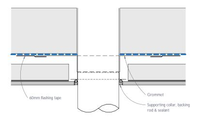
Figure 28: Pipe penetration - Plan view
