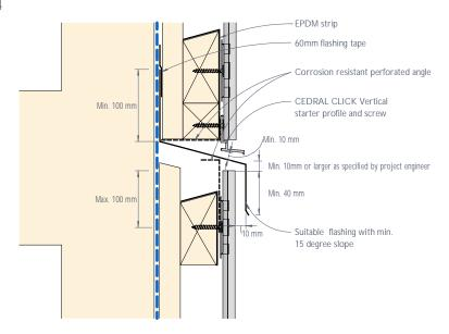
Figure 8: CEDRAL CLICK horizontal control joint and inter-storey detail
