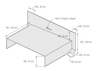
Figure 35: Corrosion resistant saddle flashing
