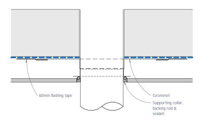
Figure 31: Pipe penetration - Plan view
