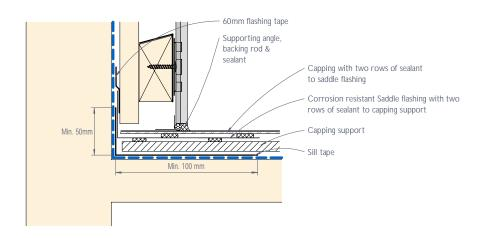
Figure 34: CEDRAL CLICK parapet junction - Section
