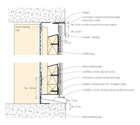
Figure 23: CEDRAL CLICK junction with exposed concrete slab or beam - Cladding flush
