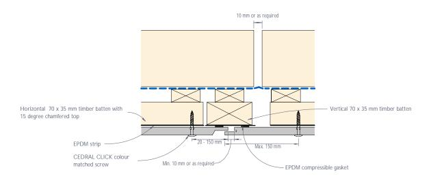
Figure 4: CEDRAL CLICK vertical control joint - Detail 1
