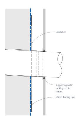
Figure 33: Pipe penetration - Section
