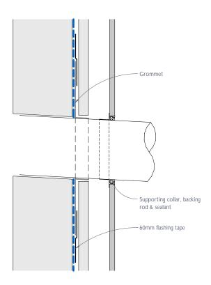
Figure 30: Pipe penetration - Section
