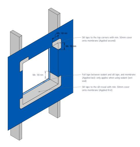
Figure 15: Isometric view of window/meter box opening - Tape application
