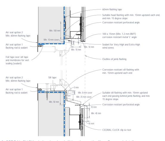
Figure 8: CEDRAL CLICK window head and sill junction or the like - Recessed detail
