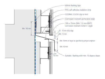
Figure 7: CEDRAL CLICK horizontal control joint and inter-storey detail
