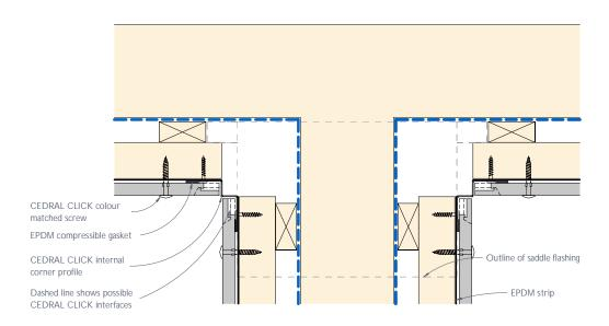
Figure 35: Parapet junction - Plan view
