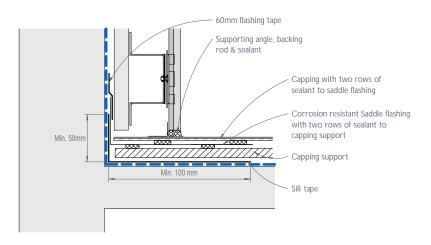
Figure 33: CEDRAL CLICK parapet junction - Section
