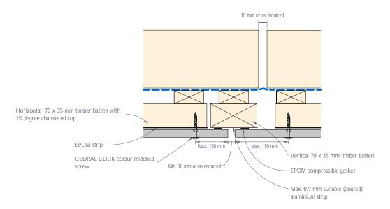
Figure 5: CEDRAL CLICK vertical control joint - Detail 2
