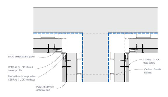
Figure 34: Parapet junction - Plan view
