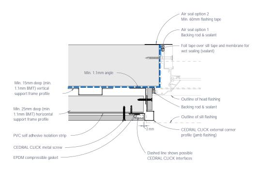
Figure 9: CEDRAL CLICK window jamb junction or the like - Recessed detail
