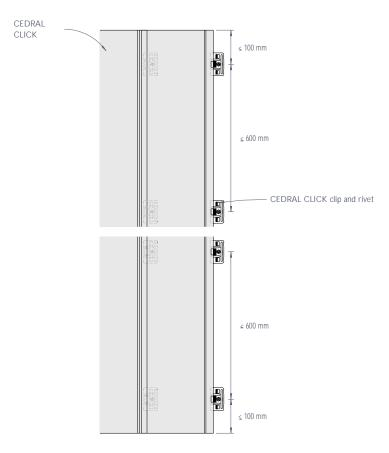
Figure 1: CEDRAL CLICK fixings arrangement - Elevation
