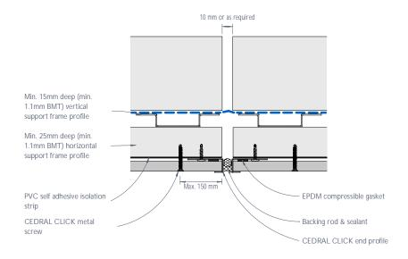
Figure 5: CEDRAL CLICK vertical control joint - Detail 2
