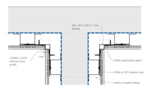
Figure 37: Parapet junction - Plan view
