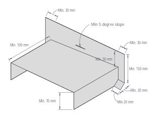
Figure 38: Corrosion resistant saddle flashing
