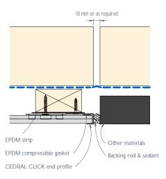
Figure 7: CEDRAL CLICK vertical control joint - Detail 3
