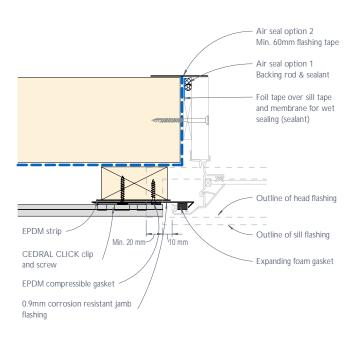
Figure 13: CEDRAL CLICK window jamb junction or the like - Flush detail
