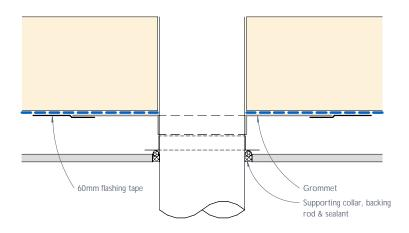
Figure 31: Pipe penetration - Plan view
