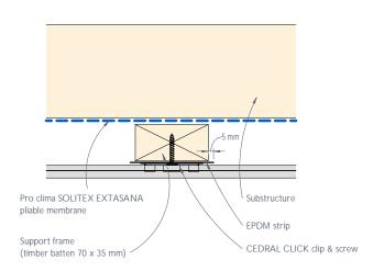
Figure 3: CEDRAL CLICK Intermediate fixing detail - Plan view
