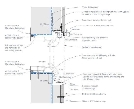
Figure 9: CEDRAL CLICK window head and sill junction or the like - Recessed detail
