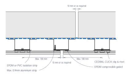
Figure 6: CEDRAL CLICK vertical control joint - Detail 2
