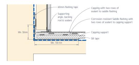
Figure 36: CEDRAL CLICK parapet junction - Section
