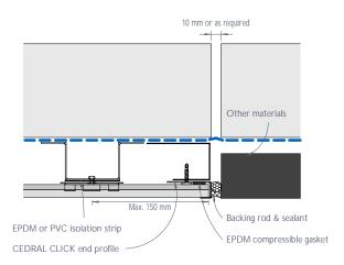
Figure 7: CEDRAL CLICK vertical control joint - Detail 3
