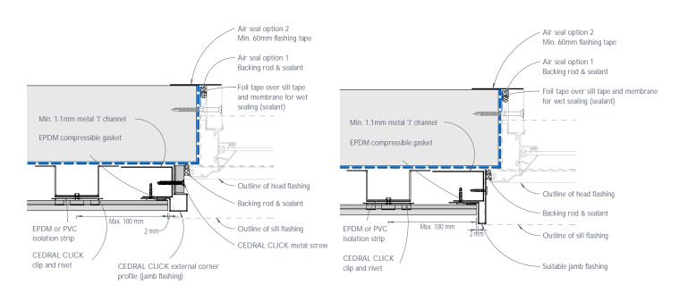
Figure 10: CEDRAL CLICK window jamb junction or the like - Recessed detail option 1
