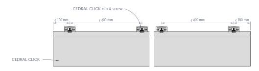
Figure 1: CEDRAL CLICK fixings arrangement - Elevation
