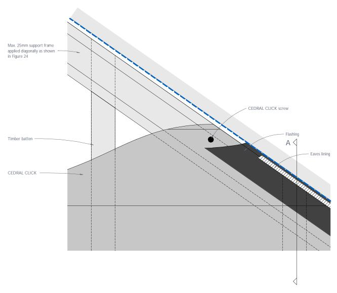
Figure 23: CEDRAL CLICK junction with angled eave - Elevation
