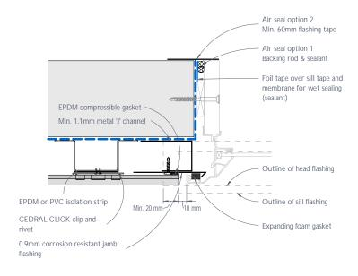
Figure 13: CEDRAL CLICK window jamb junction or the like - Flush detail
