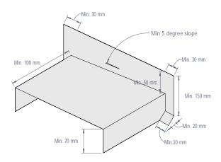
Figure 38: Corrosion resistant saddle flashing
