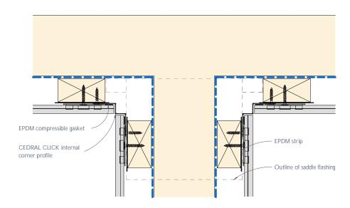
Figure 37: Parapet junction - Plan view
