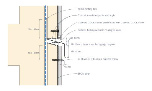
Figure 8: CEDRAL CLICK horizontal control joint and inter-storey detail
