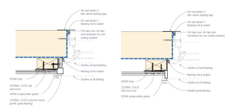
Figure 10: CEDRAL CLICK window jamb junction or the like Recessed detail option 1
