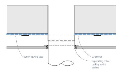
Figure 31: Pipe penetration - Plan view
