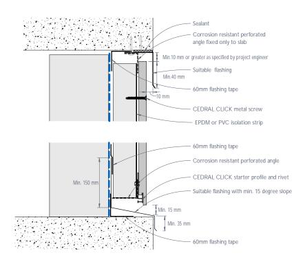
Figure 25: CEDRAL CLICK junction with exposed concrete slab or beam - Cladding flush
