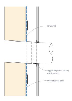
Figure 33: Pipe penetration - Section
