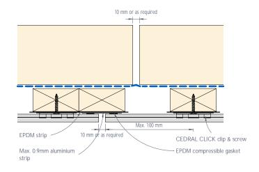
Figure 6: CEDRAL CLICK vertical control joint - Detail 2
