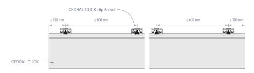
Figure 1: CEDRAL CLICK fixings arrangement - Elevation
