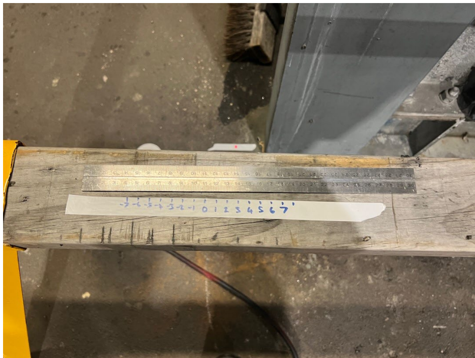
Figure 7: Elevated scale for measuring the seismic displacement with a laser
