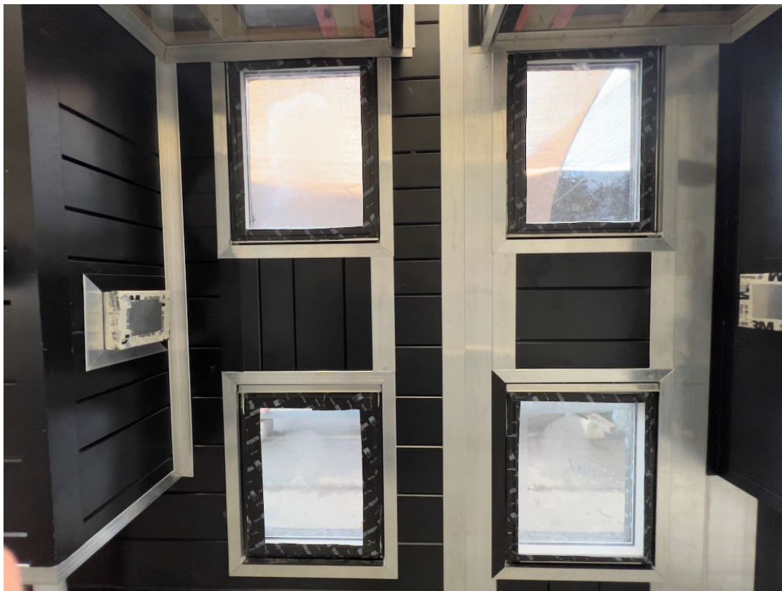
Figure 1: Photo of centre of 'wet side' of sample prior to testing
