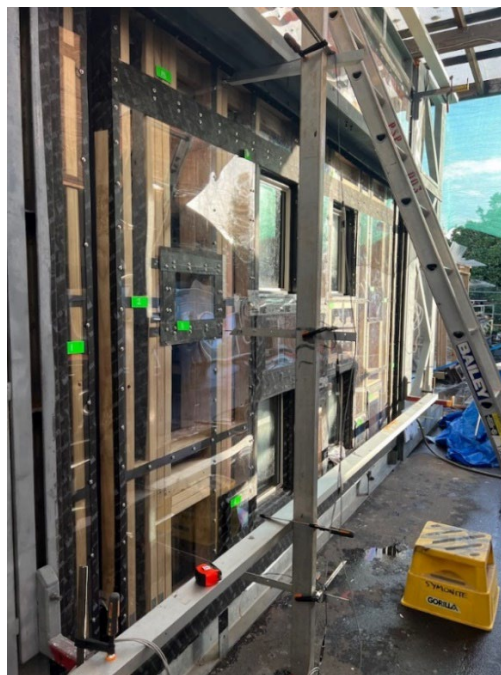
Figure 6: SLS displacement transducers on stud
