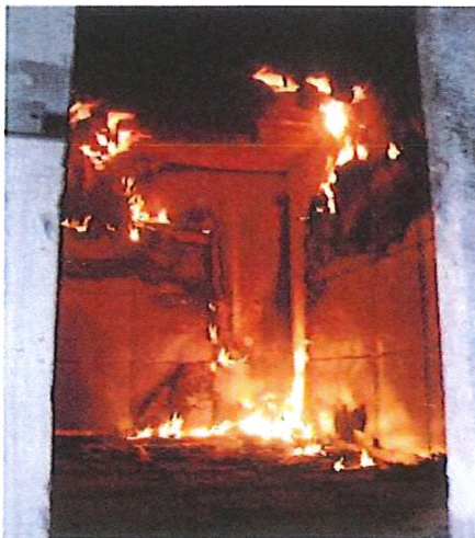
Fire in room corner test according to ISO 9705
