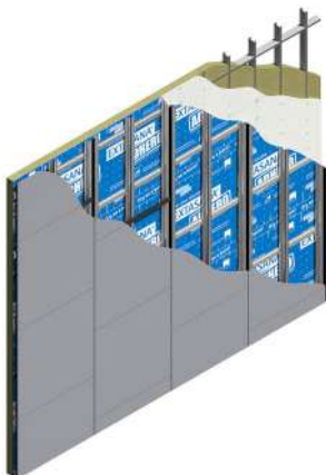
Isometric view of double layer top hat construction
