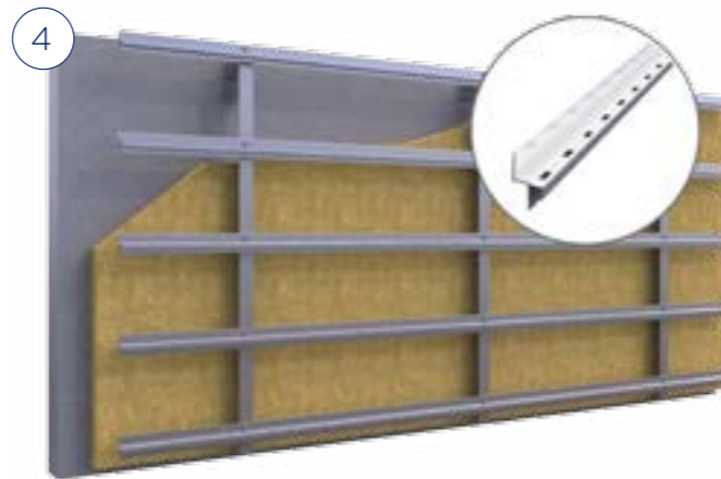
Fastening the CUPACLAD® 201 Vanguard horizontal profiles
